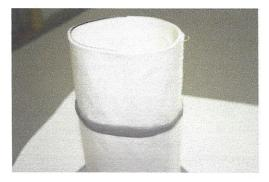
Note: Adeka Ultra Seal P-201® was used around the full outside circumference of the host pipe and between the main CIPP to seal potential exit points of water tracking through annular spaces and to ensure a water tight LPA.
